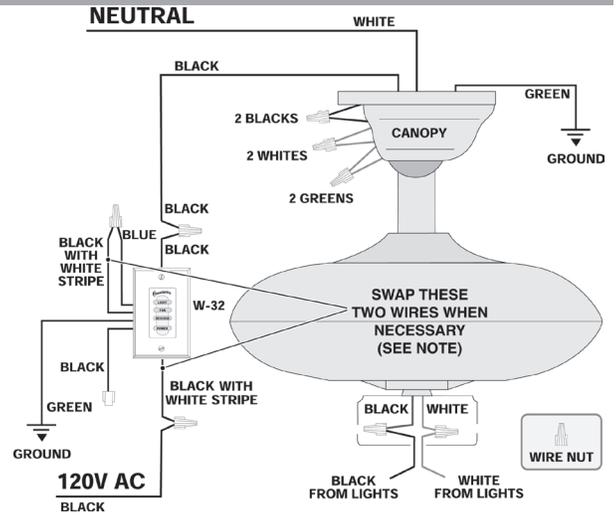
**NOTE:** This product has been evaluated and is suitable for Solid State Speed Controls.
